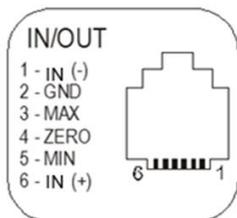
Outputs MAX and ZERO: Equivalent (common GND)
