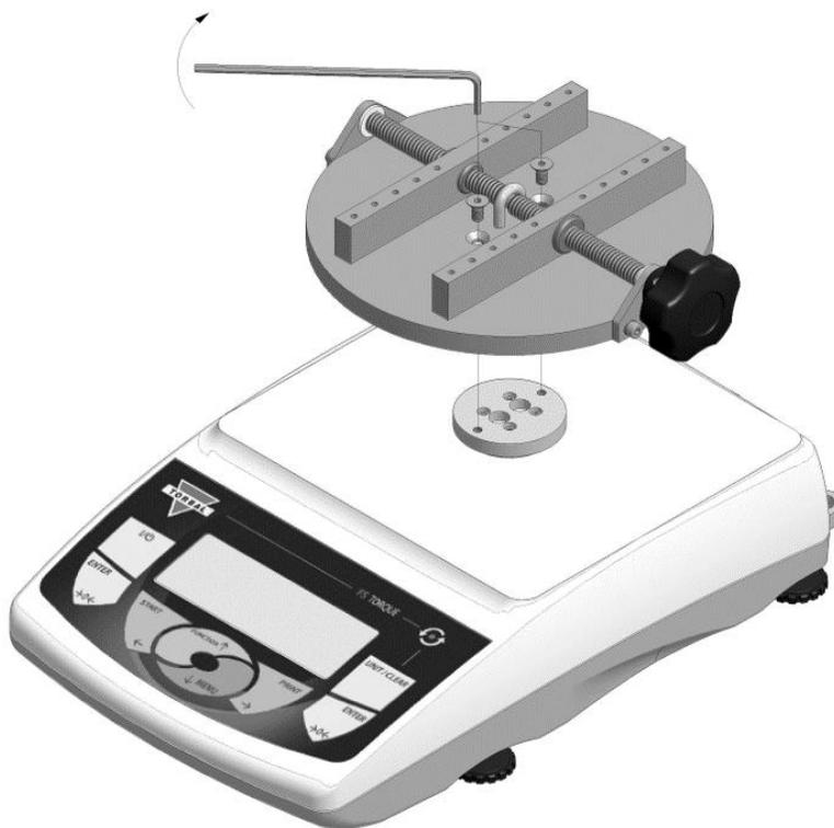
2. Use the supplied hex key to firmly connect the fixture plate to the loadcell.
